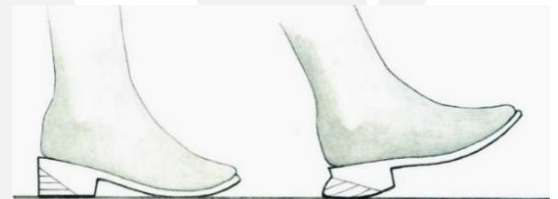
A shoe with a stiff heel can be adjusted by changing the rear part to a soft material.
